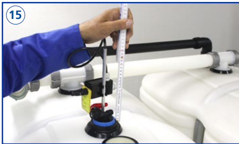
Check the limit encoder setting (y-measure).
