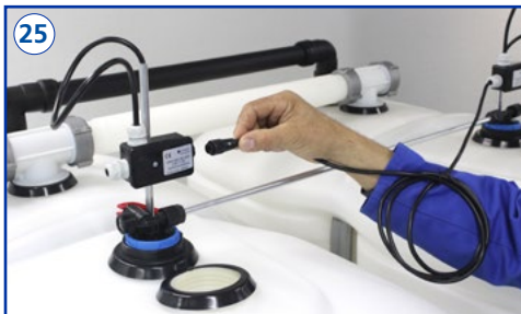
Connect the float switch of the extraction extension unit with the limit switch of the basic sampling unit.
