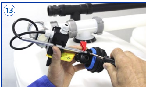
13 Fix the set GWG dimension with the screw fix.
