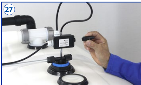
Mount the terminating plug (see no. 16) on the last extension unit.
