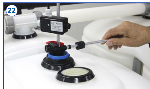
Insert the connection line into the sampling extension unit.
