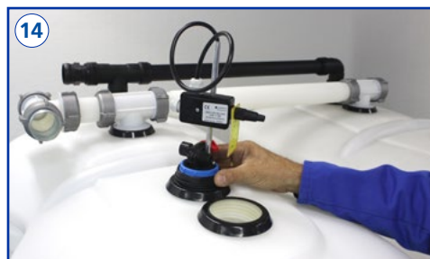
14 Screw the basic sampling unit firmly into the first tank and align it.
