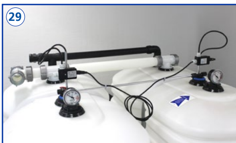
Ready assembled tank unit T102.
