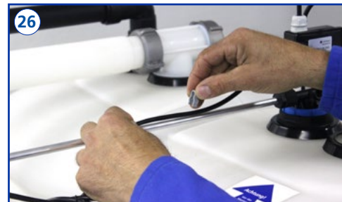
Fix the connecting cable to the sampling line with the enclosed brackets.
