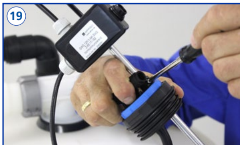
Fix the set float switch dimension with the screw.
