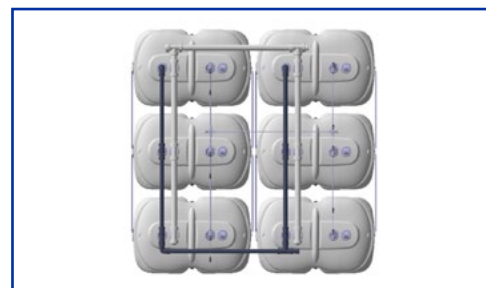
Application variant: Representation of the pipe routing on the diagram of the T 203 tank system.
