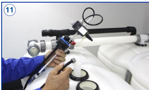
11 Lower the float and suction hose of the basic sampling unit into the first tank.
